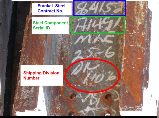
Photo of a marked column end shot by John L. Gross (NIST) for FEMA/ASCE WTC BPS (Oct. 2001 - May 2002). Taken on October 9th, 2001 (name of photo folder) at a scrap yard. Source: 911datasets.org / International_Center_for_911_Studies_NIST_FOIA / Release_37 / Release_37 / 42A0525 - G38D4 / WTCI-63-FEMA / CD1 / jlg9Oct / P1010069.JPG
